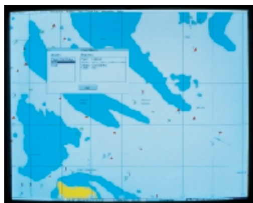
Use of the cursor query function allows quick readout of any selected chart object.
